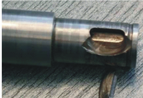
Shaft Keyway Crack
